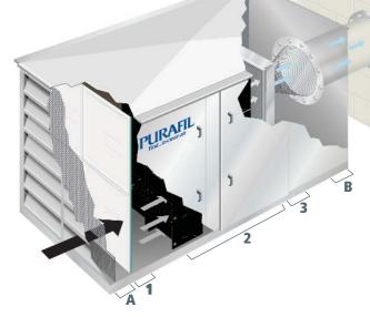
Air enters the CIF through the rainlouver with the bird screen (A). Air moves through the low efficiency particulate filter (1). Two or three passes of chemical filtration (2) are then used to remove contaminants from the air stream. The last stage of filtration is a high efficiency final filter (3). The CIF unit connects to the compressor with Outlet Plenum (B).
