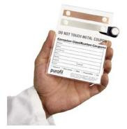
**The Corrosion Classification Coupon + (CCC+)** measures the amount of corrosion formation on copper and silver surfaces and logs the temperature and relative humidity of the immediate environment. This provides data allowing an industry standard classification of the amount of corrosion present as well as identifying contaminant classes.
