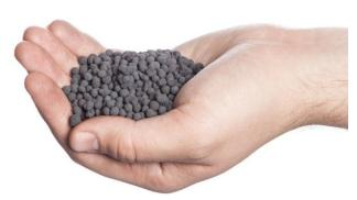
**Purafil CSO Media** has been specially engineered with a high reserve alkalinity thus assuring the best overall performance. The chemisorptive process removes contaminant gases by means of adsorption, absorption, and chemical reaction (neutralization). Harmful gases are trapped within the pellet and converted into harmless solids which remain in the pellet, eliminating the possibility of desorption and release back into the environment.
