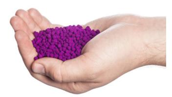
Odoroxidant SP Media has been specially engineered to provide the highest oxidation potential available thus assuring the highest overall performance. The chemisorptive process removes contaminant gases by means of adsorption, absorption, and chemical reaction (oxidation). Harmful gases are trapped within the pellet and converted into harmless solids which remain in the pellet, eliminating the possibility of desorption and release back into the environment.
