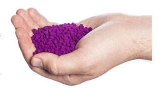
**Purafil SP Media** has been specially engineered to provide the highest oxidation potential available thus assuring the highest overall performance. The chemisorptive process removes contaminant gases by means of adsorption, and chemical reaction (oxidation). Harmful gases are trapped within the pellet and converted into harmless solids which remain in the pellet, eliminating the possibility of desorption and release back into the environment.
